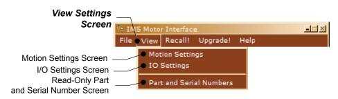
Figure 2.6.3: SPI Motor Interface View Menu
